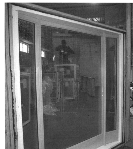
Fig. 6. Mock-up of typical fourth-floor steel-frame glass wall at the testing laboratory, photograph 2007.
